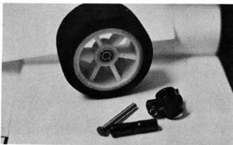
Stub axle assembly and ball-raced wheel
