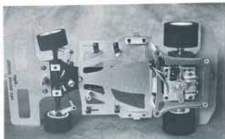
Top view of chassis showing the variable castor angle front axle beam.
